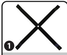
To set-up the Cross Base, place the legs perpendicular to each other in the shape of an X.
