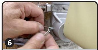
Thread the retainer rings through the hole in the end of each of the clevis pins.
