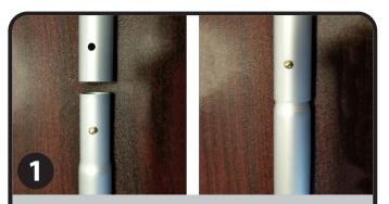
Remove foil tie from pole. For use with flags with heading and grommets, you may wish to slide the EZ-mount ring onto the top pole prior to assembling 2-piece flagpole. Line up hole of top pole section with button on bottom pole section. Depress button and slide top pole down until poles are locked together.
