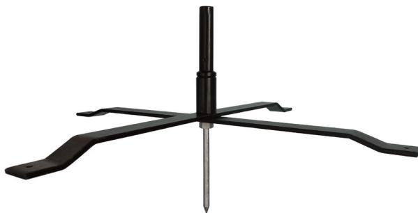
If the Cross Base will be used outside, secure the ground spike to the middle of the Cross Base. Then stick the spike into the ground and use the L-shaped stakes to secure the legs by driving the stakes through the smaller holes at the ends of the feet.
