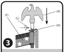
Slide the finial (A) (Eagle, Cross or Spear) over the top of the pole (H). Screw brass screw (B) through the pole (H) using a Phillips head screwdriver to secure.
