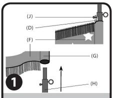
Find the open "pocket" or "sleeve" (G) at the back edge of the flag (F). Slide the flag sleeve (G) up the top flagpole section (H), top edge first, until the top of the flag reaches the brass screw (J). Find the Leather tab (D) at the top of the flag sleeve (G) and slip it onto the head of the brass screw (J) to hold the flag in place.
