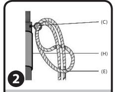
Affix the tassel (E) cord to the screw eye (C) as shown in the drawing:
