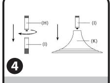
Screw bottom pole (I) to top (H). Place completed assembly in stand (K).
